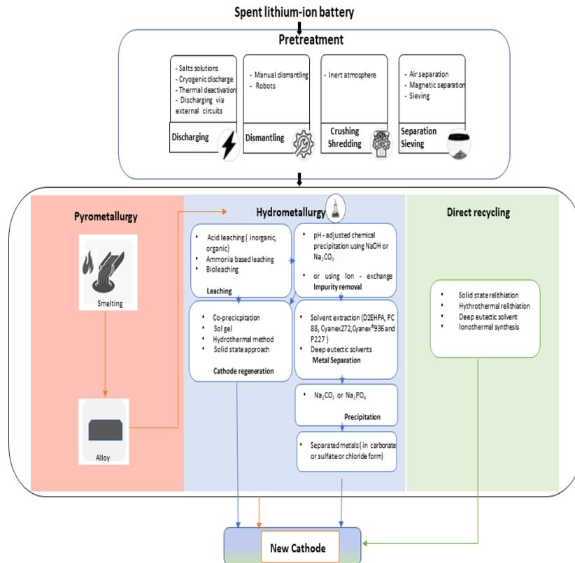
Figure 10 General recycling processes for lithium-ion batteries
