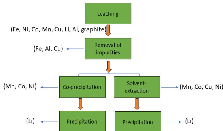
Figure 12 Example of hydrometallurgical processing
