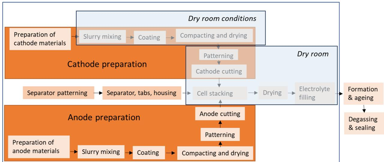
Figure 2 Conventional cell manufacturing details. In BatWoMan, stack drying, electrolyte filling and slurry mixing will not be carried out under dry room conditions.
