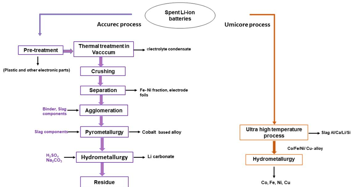
Figure 11 Flow sheet of Accurec and Umicore recycling processes.
